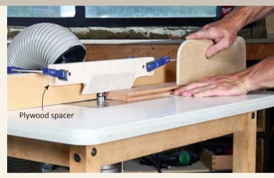
**Rout the tongue in one pass.** Keep the pressure steady by bumping out the featherboard with screws and plywood spacers to clear the taller cutter. Use a pushstick as before for a smooth tongue with a consistent thickness and width.
