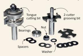
Mating bits for efficiency and accuracy. This 2-piece set from Freud accommodates stock thicknesses from 1/2" to 11/4". One of the bits cuts the tongue, and the other the groove. You can fine-tune the cut on both bits by adding or subtracting spacers.
