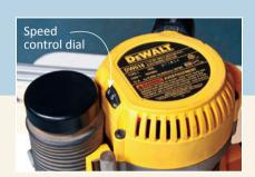
**Dial it down.** Use a variable-speed router, and keep your speed around 15,000 RPM to lower vibration and reduce stress on the router and bit.
