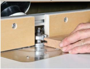
**Eyeball the height.** Set the tongue bit's height by lining up its cutting edges with the groove, and then make a test cut in scrap to verify your setting.
