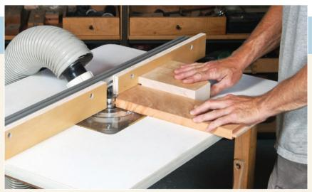
Back it with a block. Use a squared pushblock to keep the workpiece steady against the bit's bearing and the fences while you rout, and to prevent tearout at the back.
