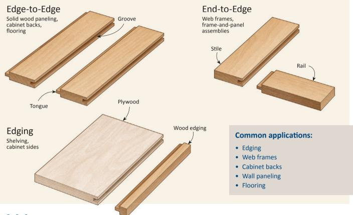
With its relatively short tongue that fits into a shallow groove, the tongue-and-groove joint is woodworking's diminutive cousin to the mortise-and-tenon. Thankfully, it's much easier to make, in large part due to modern routers and router bits. The shorter tongue is a good choice for registering parts, such as when fitting wood panels or boards for cabinet backs and flooring (in which case the joint is typically assembled without glue.)
