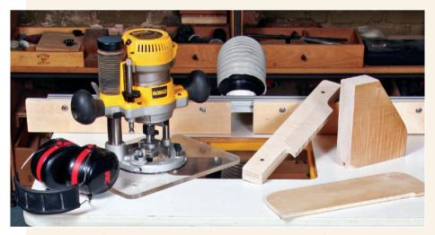
**The right stuff.** For tight, crisp joints, equip your table with a  $1\frac{1}{2}$  hp (or more) variable-speed router, a split fence, a featherboard, a hefty pushblock, a plywood pushstick, and through-the-fence dust collection.
